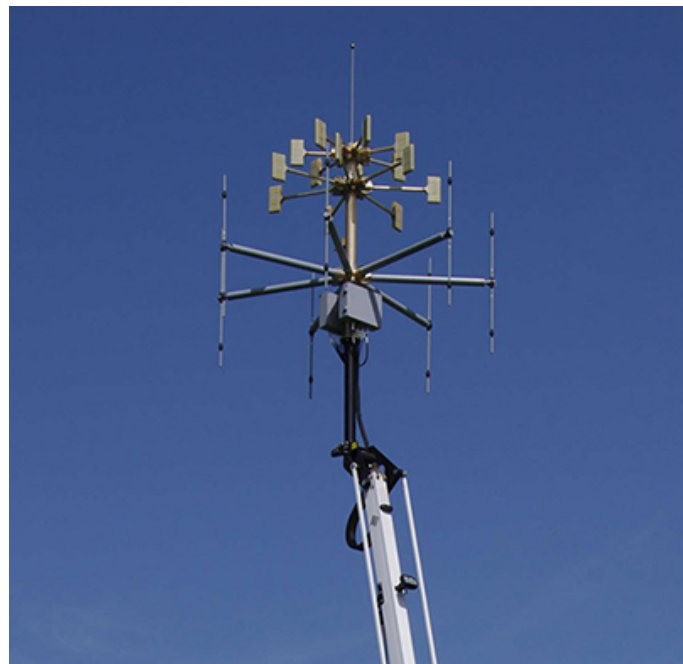
Figure 4-2: The Antenna Array of the Passive Radar Demonstrator Produced by Airbus Space and Defence.
